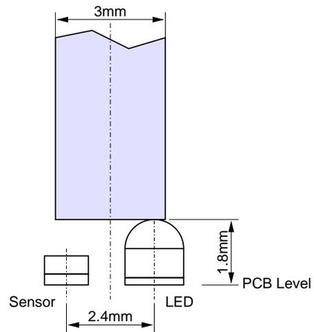
Fig. 5: Mechanical Dimensions of the Setup
