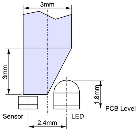
Fig. 10: Mechanical Dimensions of the beveled Setup
