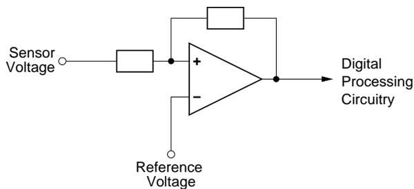
Fig. 3: Most simple Analog Hardware
